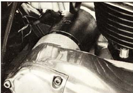
Lucas electric starter drives Bonneville crank through 20:1 gear reduction in right case cover.
