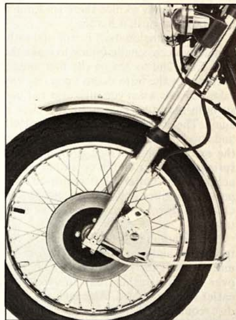
Triumph front forks are too stiffly sprung, as is rear swing arm. High quality chrome abounds on headlight, fender and trim. Polished spoked wheels are made in Italy.
