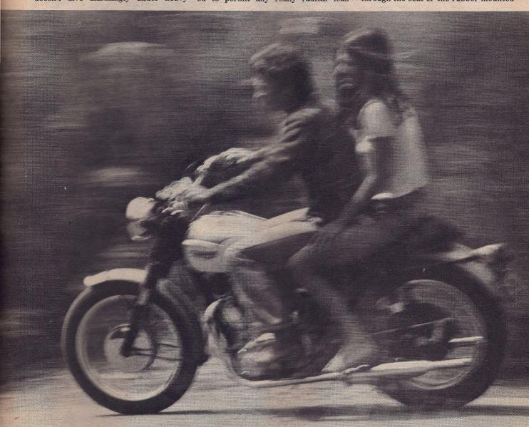
braking. But while its compression response works well enough, there seems to be insufficient rebound damping for choppy surfaces. Combined with the stiff action and limited travel of the Girling shocks, the Triumph can be thrown into a serious wobble in rippled turns. And in freeway riding the suspension develops a hobby horse action on the expansion joints at speeds below 60.
