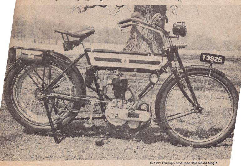
In 1911 Triumph produced this 500cc single speed single that had a clutch in the rear hub. The engine featured side valves and a manually operated oil pump.
