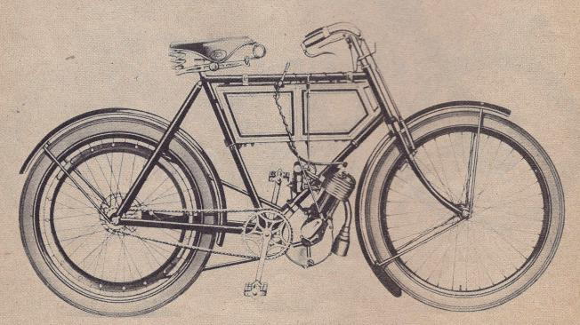
The 1903 Triumph featured pedals to start the Belgian engine. The single speeder had no clutch.
