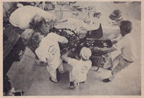
Kawasaki team mechanics, Pocono Raceway, Pennsylvania, 1972. The race sometimes takes place in the pits. Here six mechanics tear down and rebuild a complete roadracer before the next race.
