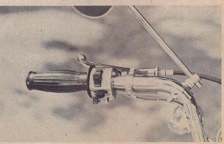
L/H handlebar has hi-lo beam, turn signals, and horn, all thumb operated. Clutch action is adjustable for that perfect squeeze.
