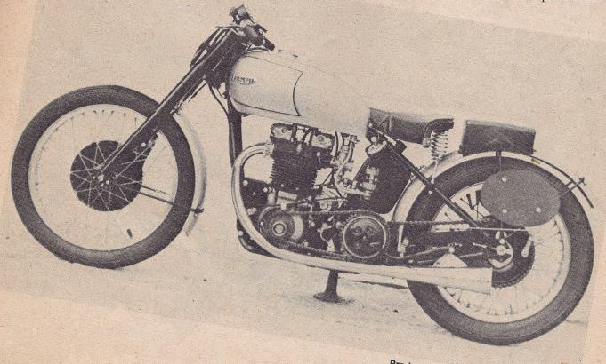
Produced in 1948, '49, and '50, the 500cc Grand Prix model featured an alloy engine, 42 HP at 6800 rpm and a speed of 112 mph. A beautiful road racer.
