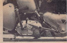
Pre-unit construction, the Thunderbird featured a separate engine and gearbox design, which was considerably heavier than the more modern unit construction, introduced in '63.
