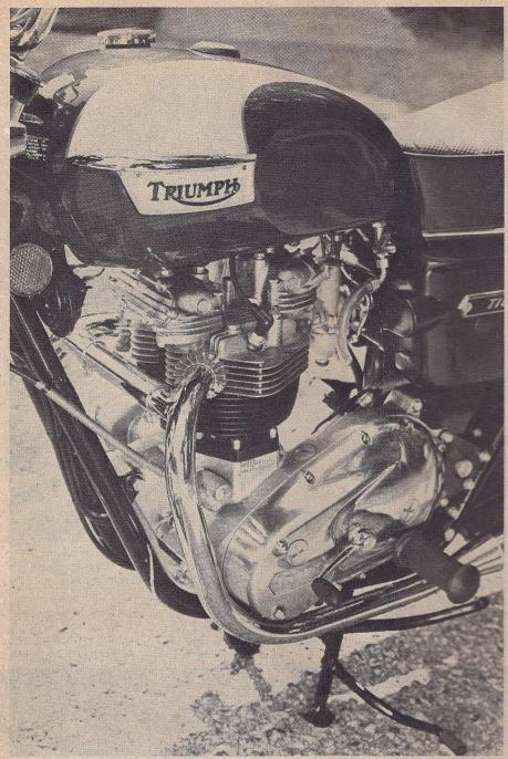
Tiger 750 powerplant employs the recently converted leftside shift, only a single 30 mm Amal carb, an exhaust balance tube, and for cosmetics the side cases are bright polished aluminum.
