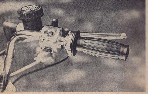
R/H, handlebar cushion grips reduce vibration; the Lucas switches for electric start are not functional.
