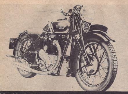
A dismal failure, the 1935 vertical twin had a hand shift in an era when the other British bikes all had a foot shift.
