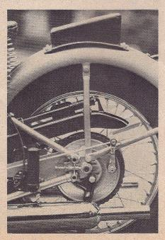
No hydraulic damping was used in the Thunderbird's unique rear suspension. The rigid frame models were, at this point, fading fast, as they were not as comfortable as the newer sprung hub model. Travel was here limited to  $2\frac{1}{2}$  inches.
