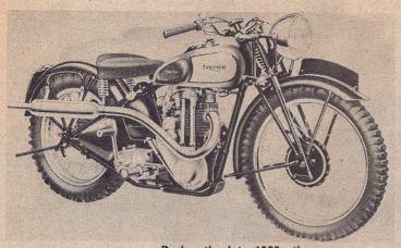
During the late 1930s the company produced good 250, 350 and 500cc singles which could be had in trials trim with knobby tires, a 21 inch front wheel and wide ratio gears.
