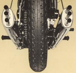
Power as never before in a production motorcycle is no idle boast. During development, it was found that standard road tires were not suitable. So an entirely new concept in tire design and tread pattern had to be developed. The result is a brand new tire, semi-triangular in section with a specially developed buttressed tread pattern. This tire the Dunlop K81 combines long life with safety all-angle road holding characteristics.
