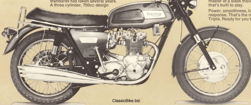
Advanced design, all-alloy, 45 cu. in., three cylinder power plant.
