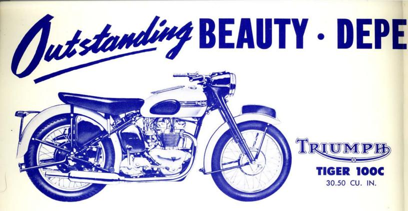
This model has been produced for the Tiger 100 enthusiast who intends to use his machine for racing. The specification is similar to that of the Tiger 100, but includes twin Amal carburetors with remote float bowl, high compression pistons, racing camshafts, twin rotor twist grip and a 1-gallon oil tank. All moving parts of the engine are highly polished and a really exceptional performance, in racing trim,
