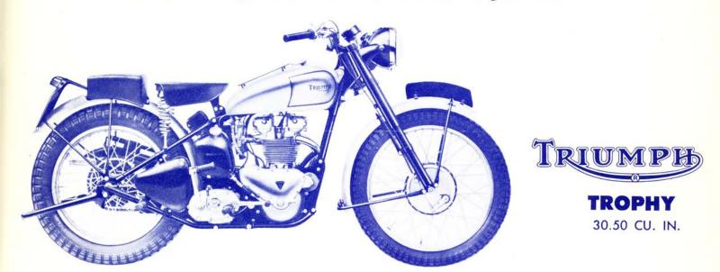
A light, fast motorcycle designed from stem to stern for the competition rider. All alloy engine,  $2\frac{1}{2}$  gallon gasoline tank, wide clearance aluminum mudguards,  $70^{\circ}$  steering lock, two-in-one exhaust, wide ratio gears, 400—19 rear and 300—20 front tires, quickly detachable headlamp and many other special
