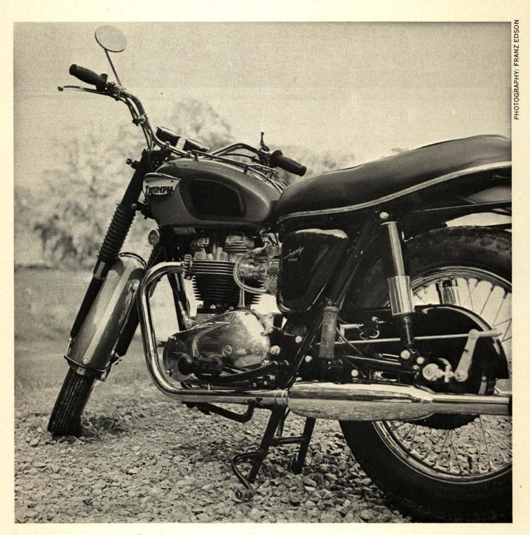
"British Twin"—parallel cylinders with overhead valve actuation by pushrods and gear-driven camshafts mounted high in the cases. The crankshaft is a bolt-up unit with a single, central flywheel and two mainbearings at the outer ends. The crank journals are positioned together (pistons rise and fall simultaneously, cylinders fire alternately) and plain automotive-type shell bearings are used at the lower ends.
