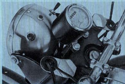
Compact headlamp assembly with main beam warning light and quick action switches
