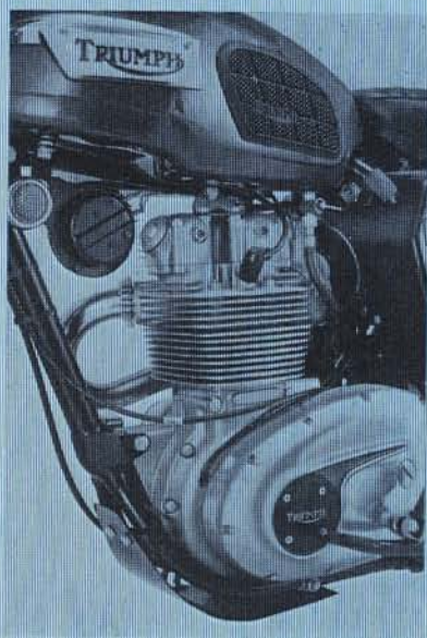
Sleek square finned engine unit develops 22 b.h.p. at 8250 r.p.m.
