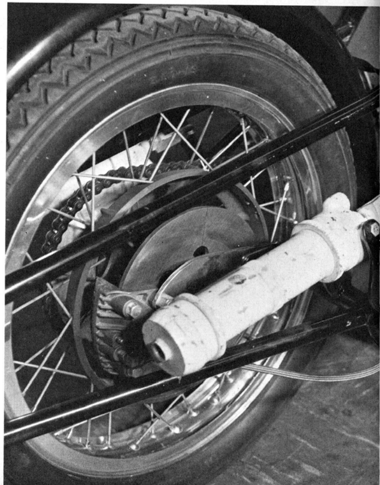
Rear wheel section has Al Gunter magnesium rear wheel hub with Borrani WM3-19" Alloy Rim, Airheart disc brake, hydraulically operated by pedal. Retractable skids are pneumatically actuated by two way valve for starting and stopping X-1.
