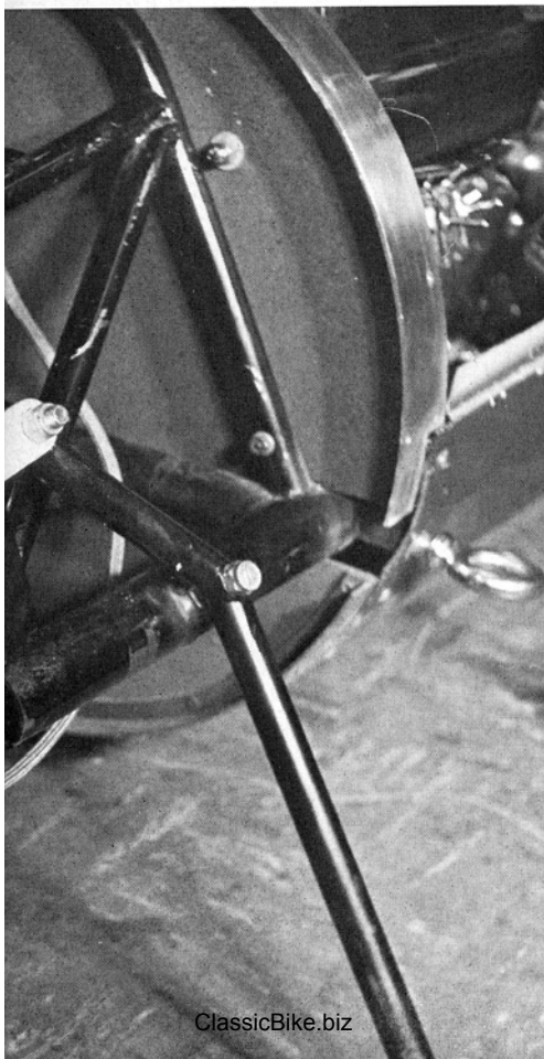
Overhead view of rear wheel section and engine compartment. Note sturdy roll bar at top of picture. Projecting eyebolts aid lifting and transporting, are quickly removable for running. Fender keeps salt from engines.
