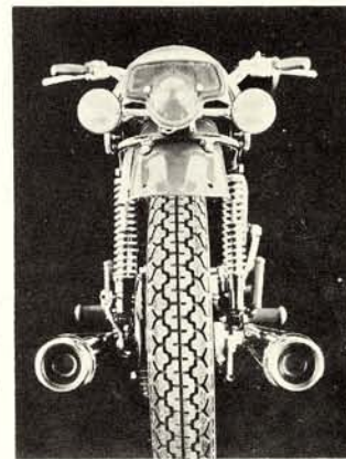
Girling rear shocks couple chrome plated springs with hydraulically-dampened cylinders for smoother riding.
