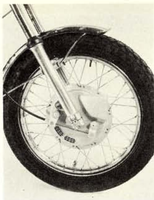
Newly designed brakes, ride lighter, stop surer. New air scoop keeps front cooler.
