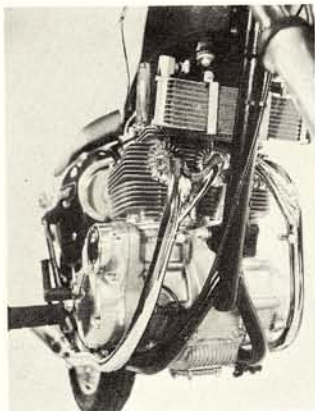
Triple carbs and triple cylinders thrust 45 ft. lb. of torque @ 6900 rpm.
