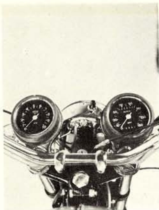
Speedo-tach packs are rubber-mounted to absorb shock, angled for easy reading.
