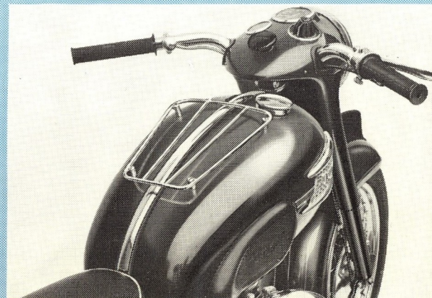
The new petrol tank featured on the 650 c.c. range is of pleasing shape and has a comfortable capacity of 4 gallons (TR6 3 gallons). It is easily removed when required and has the ever useful parcel grid on top and handsome Triumph motifs on each side.
