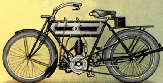
1906 3 HP with magneto ignition.
