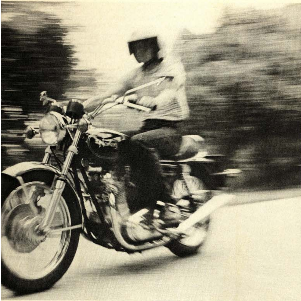
Rear brake is cable actuated, centerstand is well tucked in for cornering clearance.
