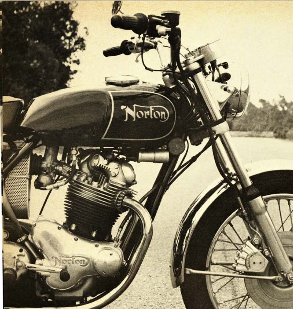
The double damping forks, dubbed the Roadholders by Norton, are an exclusive feature of the Commando.
