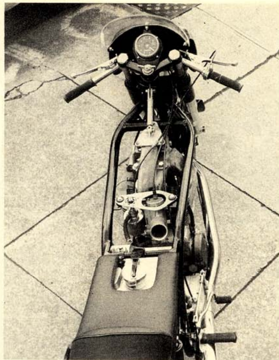
With the tank removed, the huge Amal carburetor is exposed for service.
