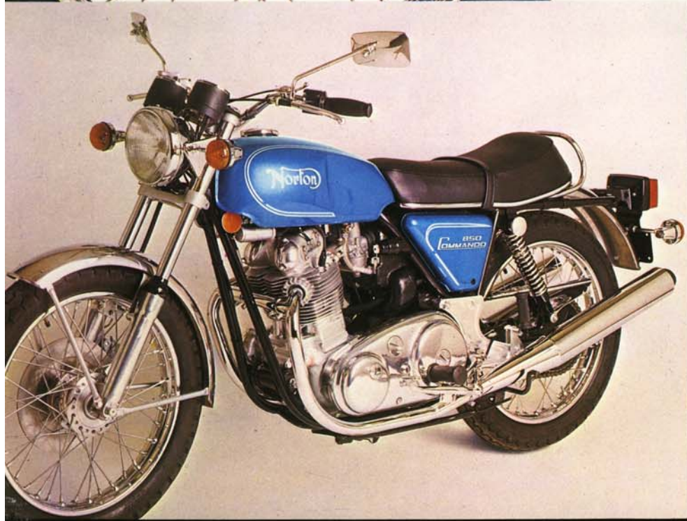
Commando 850 with low noise air intake and exhaust system including new reverse flow annular discharge muffler (Patent applied for).
